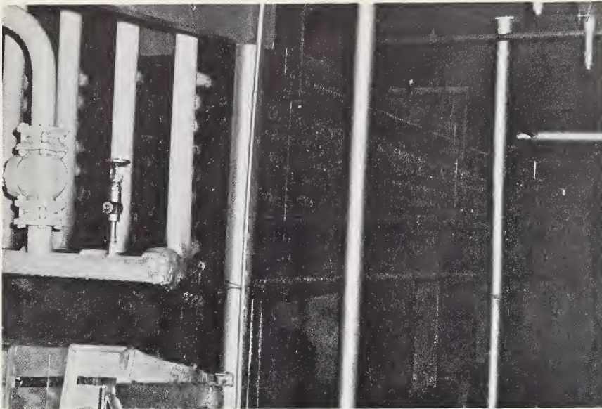
Figure 5.--Shower of water cascading over cooling coils and showering onto packed produce.
